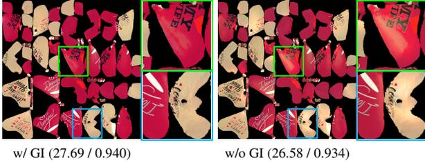
Figure 8: **Reconstructed albedo with/without GI.** We show the impact of modeling global illumination (GI) on material reconstruction. The above images are the reconstructed albedo maps with GI on/off, with their errors listed below (PSNR $\uparrow$  / SSIM $\uparrow$ ). Without GI, the optimization tends to “bake” the indirect lighting into the albedo map.
