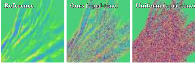
Fig. 5. Ablation: We compare variance derivatives for the Tree scene estimated using different sampling methods. In this case, the derivatives are emerge solely from the boundary component of Eq. (14).
